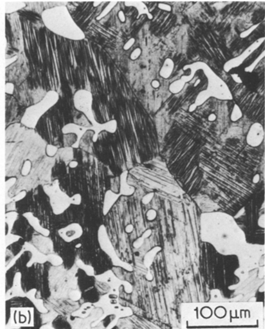
Figure 1 Alloy 1: Ni–28.75 at% Al–2.5 at% Ta. (a) Homogenized at 1260° C for 48 hours and water quenched. Banded \beta -martensite structure showing straight, parallel-sided plate morphology; some regions contain three differently orientated sets of plates, e.g. at A, B, and C, while other (smaller) regions contain only one set of plates e.g. at D. (b) Homogenized at 1350° C for 5 hours and water quenched. Shows a larger proportion of \beta -martensite structure.
