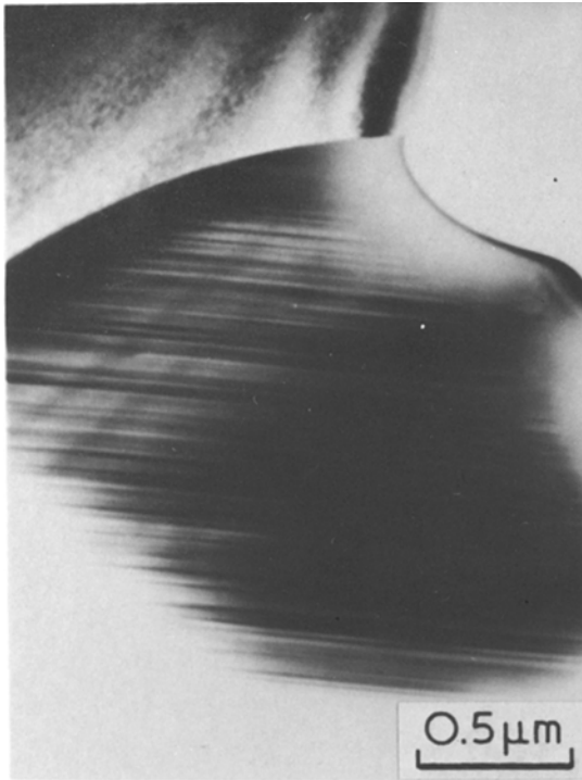
Figure 11 Alloy 5: Ni–22.5 at % Al–5.0 at % Hf; annealed at 990° C for 4 days. Fine striations within a particle of (Ni, Al) 7 Hf 2 representing faulting on the (0 0 0 1)-plane.
