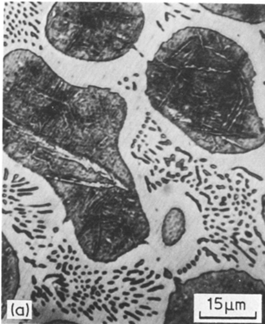
Figure 2 (a) Alloy 1: Ni–28.75 at% Al–2.5 at% Ta; as-cast. Primary \beta -phase regions (martensitic) plus eutectic regions ( \beta + \gamma' -phases). (b) Alloy 3: Ni–20.0 at% Al–7.5 at% Ta; as-cast. \gamma' + \beta -phases.
